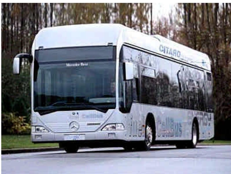
Figure 1 – The Citaro bus equipped with a Ballard fuel cell (CUTE project)
