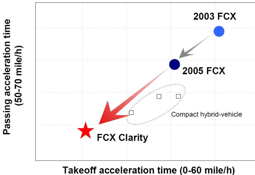
**Figure 13:** Development of the acceleration characteristics of the Honda FCX fuel cell vehicles over time (Source: Honda). Exact numbers are not published by Honda. The figure presents only relative improvements within the Honda FCX line of vehicles that are achieved by increasing experience and technological know-how over time.
