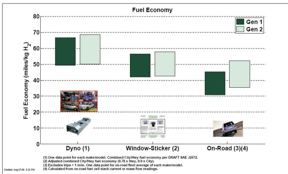
**Figure 6:** fuel economy development of vehicles in the National Fuel Cell Vehicle Learning Demonstration Project, USA. Distinction is made between laboratory measurements (Dyno), values given by the OEMs (Window-Sticker) and practice (On-Road). For conversion to liters of gasoline equivalent (lge): 30 miles/kg = 12,2 km/lge; 40 miles/kg = 16,3 km/lge; 50 miles/kg = 20 km/lge; 60 miles/kg = 24,4 km/lge; 70 miles/kg = 28,5 km/lge (Source: K. Wipke, NREL)
