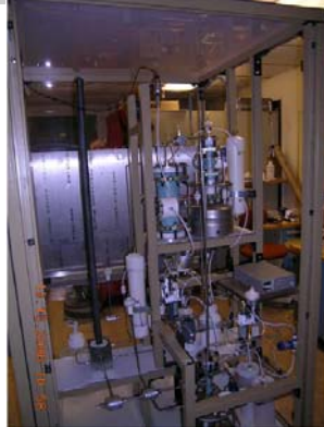
H 2 SO 4 DECOMPOSITION DEVICE
