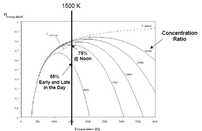
Figure 5: Solar collection efficiency. The efficiency of a solar receiver varies throughout the day because solar input is changing and thermal losses are constant. The highest efficiency occurs at noon when solar input is highest<sup>5</sup>.
