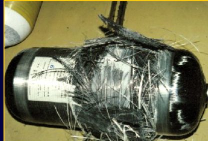
Hydraulic burst test
