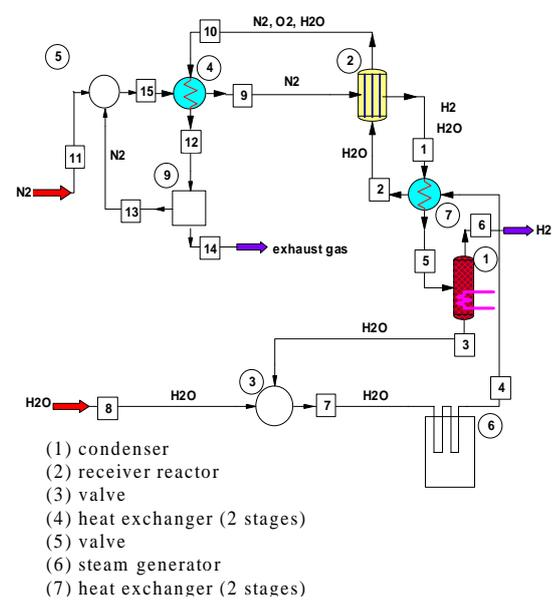
Fig 1: Basic flow sheet of water splitting process<sup>2</sup>
