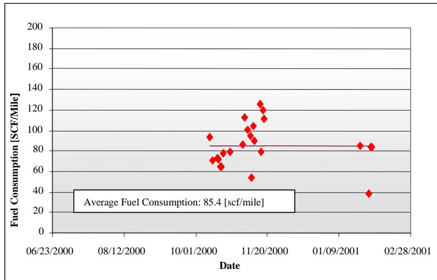
**Figure 7: Fuel consumption of ZEBUS for transit track test**
