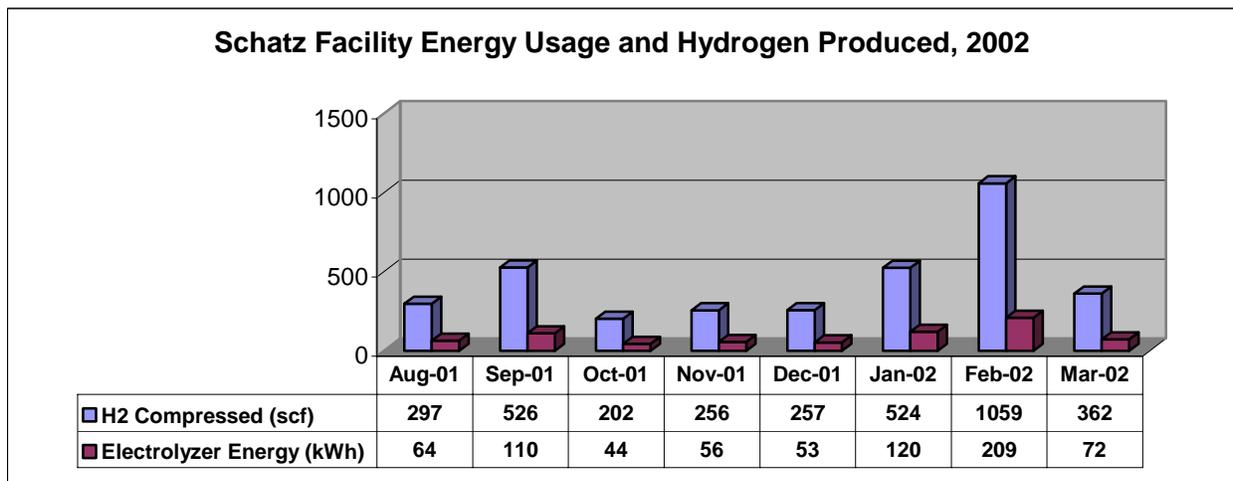
**Figure 5: Teledyne Energy Systems electrolyzer power usage and hydrogen production**
