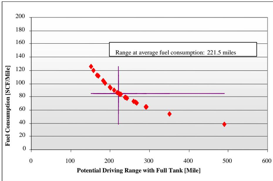
**Figure 8: Potential driving range of ZEBUS with full tank**
