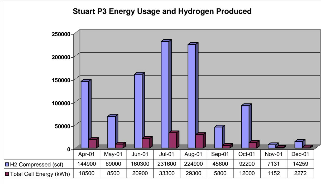
**Figure 6: Hydrogen produced using Stuart Energy Systems P3 Unit**
