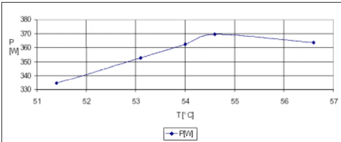
**Figure 7: Temperature behavior of the PEM Fuel Cell**
