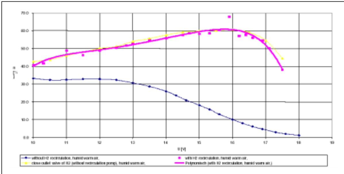
Figure 10: Fuel cell efficiency depending on the voltage
