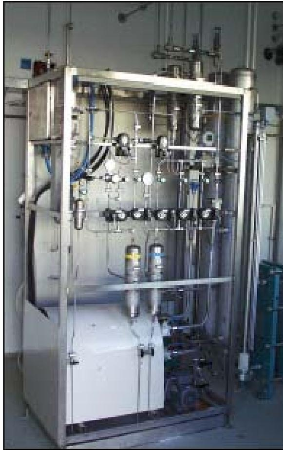
**Figure 3: 20 kW pressurized electrolyser**
