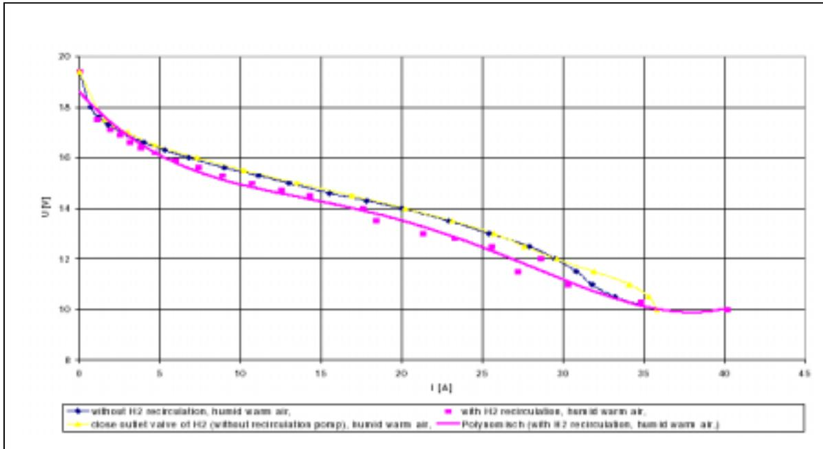
Figure 8: Voltage/current diagram of the PEM Fuel Cell
