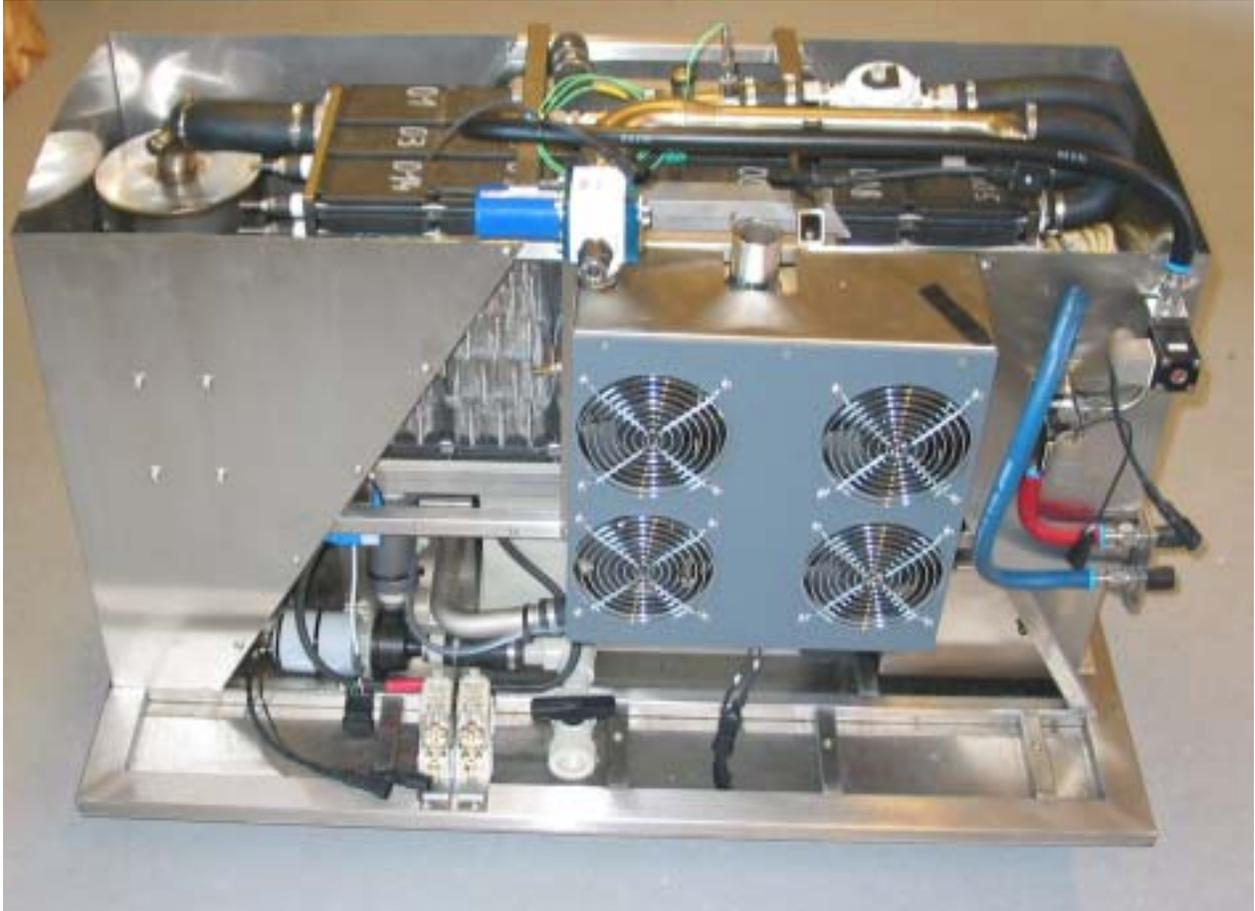
**Figure 9: The ZeTek Power fuel cell with electrolyte circulation system, CO<sub>2</sub> removal, etc.**
