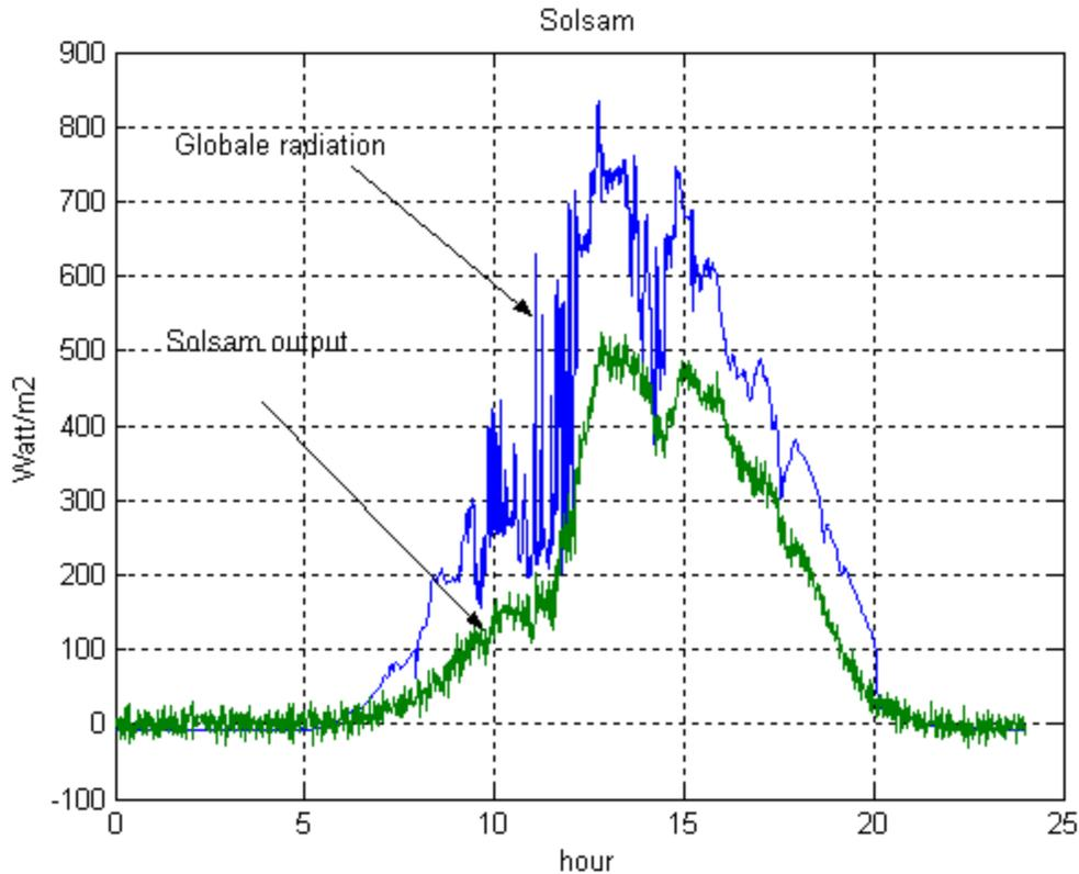
**Figure 5: Heat production from Solsam solar collectors**
