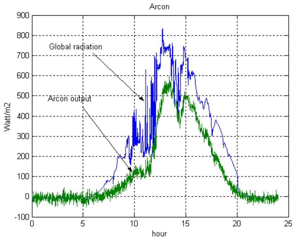
**Figure 4: Heat production from Arcon solar collectors**
