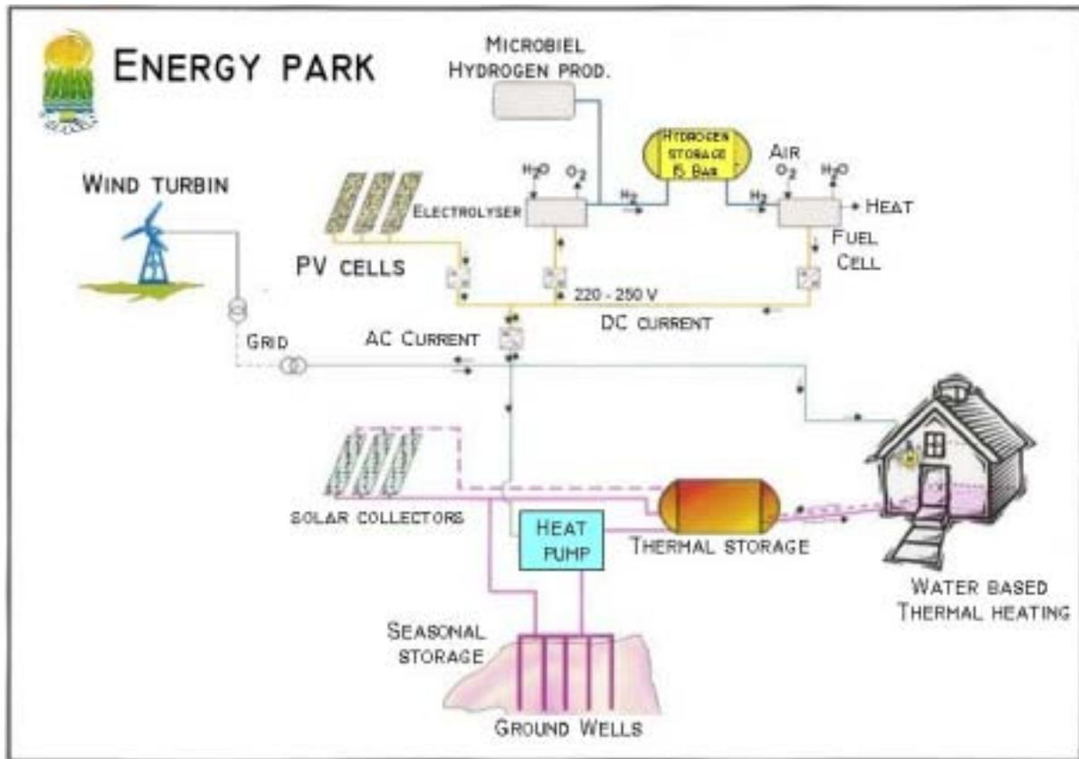
Figure 2: A schematic drawing of the Energy Park
