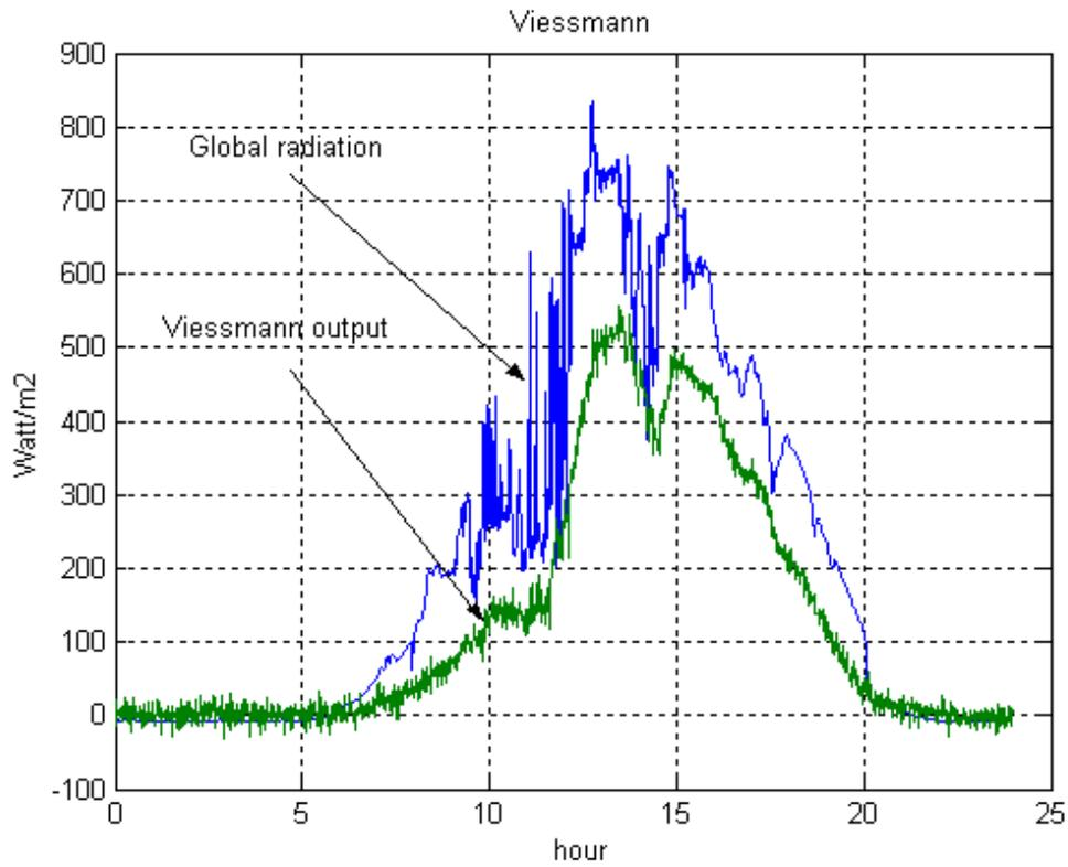
**Figure 3: Heat production from Viessman solar collectors**
