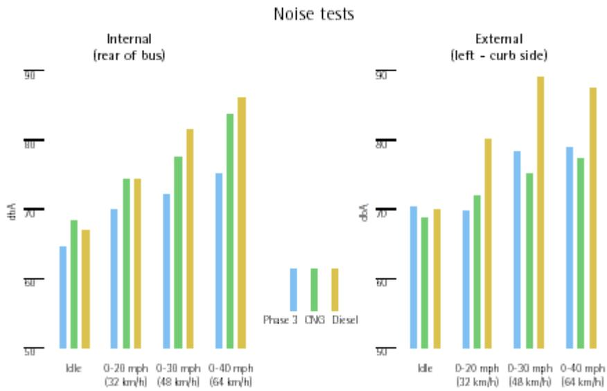
Figure 12: Noise tests
