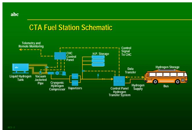
Figure 6: Schematic of the CTA hydrogen fueling facility
