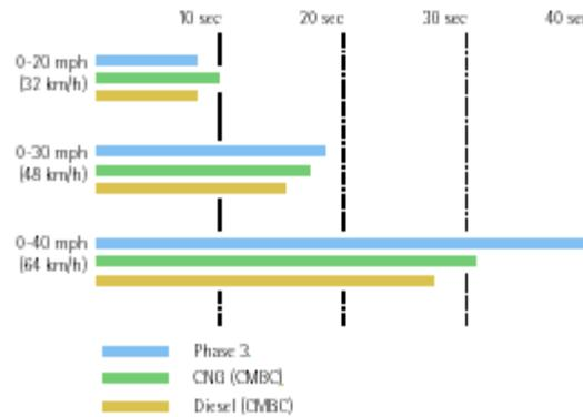
Figure 9: Acceleration from rest
