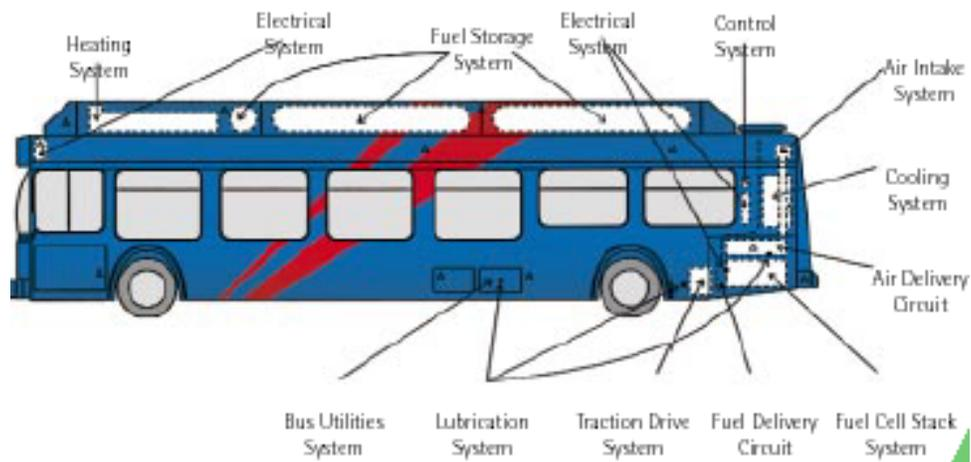
Figure 2: Schematic picture of XCELLSIS/Ballard fuel cell bus
