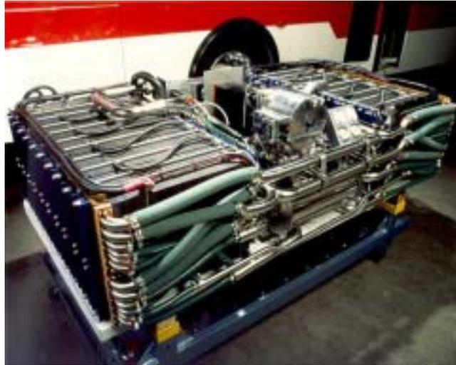
Figure 1: XCELLSIS fuel cell engine
