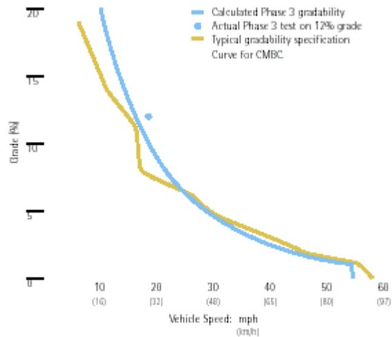
Figure 11: Typical gradability at 17 tons (15.4 tonnes)
