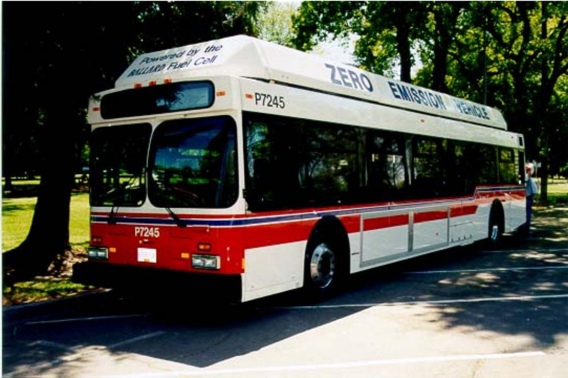
Figure 3: The Vancouver Ballard fuel cell bus
