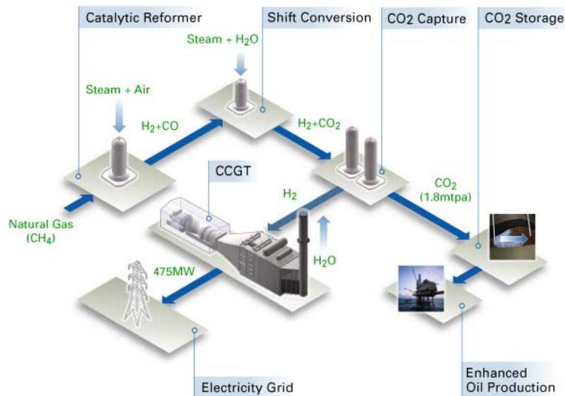
Figure 1 Diagram of the proposed hydrogen power plant at Peterhead ©BP
