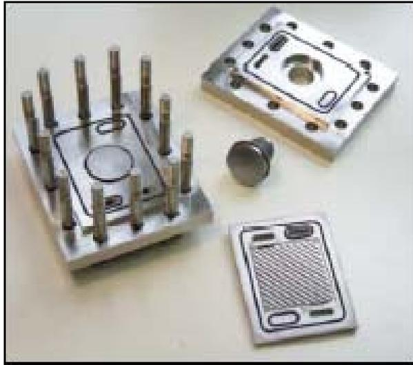
**Figure 4: Electrolyser components (Showcase 2)**
