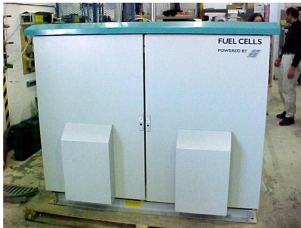
Figure 2a: The HPower FC system inside a closed enclosure
