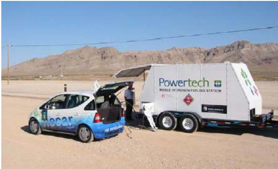
**Figure 8: Demonstration of the hydrogen mobile fueling station. This unit supported fueling of fuel cell vehicles during a road rally from Riverside, California to Las Vegas, Nevada in 2001.**
