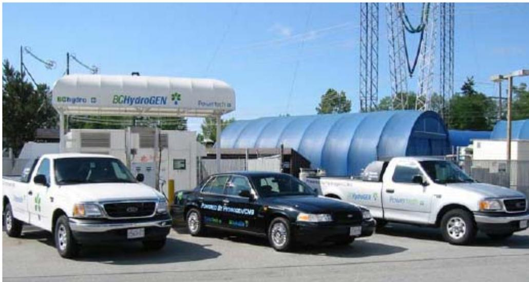
**Figure 4: ICE vehicles converted to operate on a combined CNG and hydrogen fuel (Truck: Ford F150 / Passenger vehicle: Ford Crown Victoria)**
