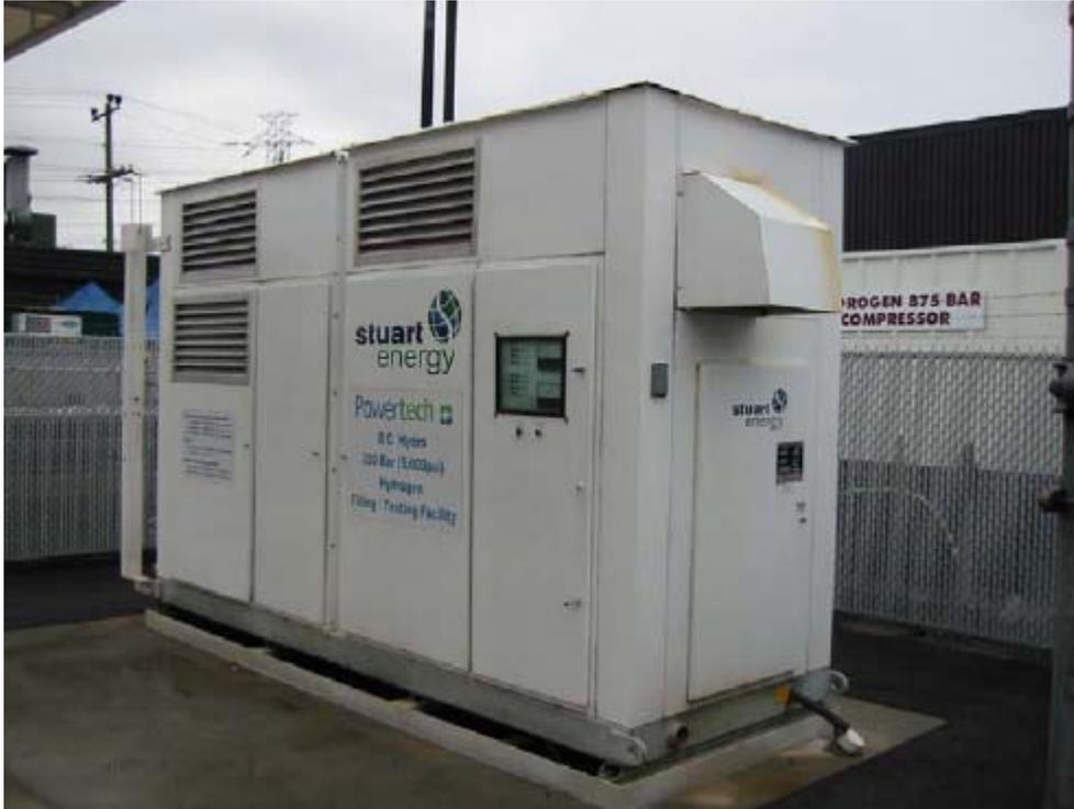
**Figure 2: Prototype electrolyser used for the CH<sub>2</sub>IP program. The package also included 2 small compressors and the equipment needed for hydrogen purification**
