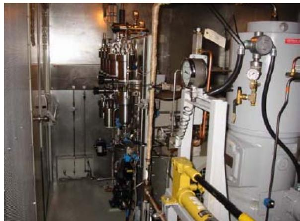
**Figure 5: The PPI Diaphragm compressor, cooling system, and purification system were housed in a container package by IMW Industries. Attached in the container is a compartment where the controls and data acquisition systems were installed.**
