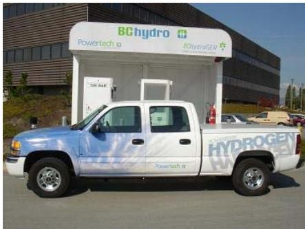
**Figure 2 Hydrogen vehicle**
