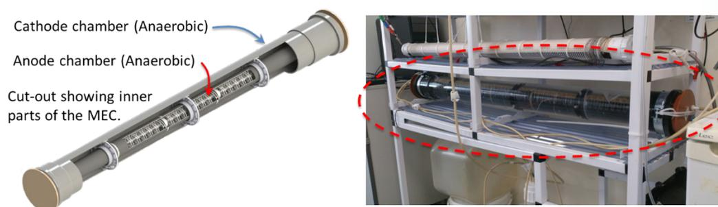
Figure 1. Schematic and photograph of a tubular microbial electrolysis cell for biohydrogen production, developed at the University of South Wales.
