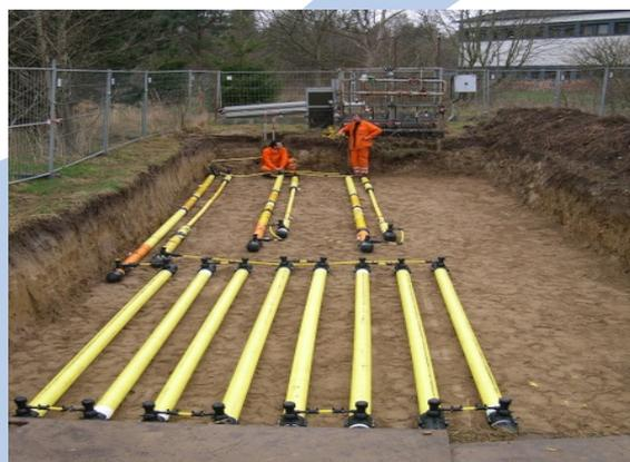
Test of polymer distribution pipes for hydrogen transportation
