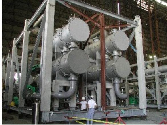
**Figure 6-2 Example of exchangers being bundled on a module with valve manifolds located at the rear of the module. The lower frame of this module was buried in the concrete slab at site.**
